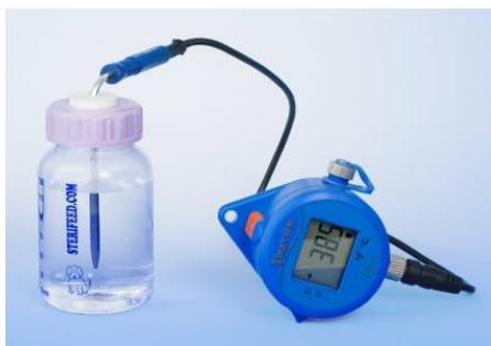
Figura 3. Data logger Tiny Tag View 2
